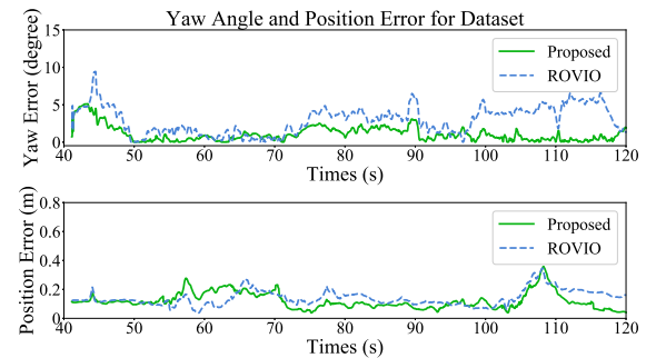
Fig. 7. Errors of position and yaw angle under ROVIO and our proposed algorithm on EuRoC-MH01. Dotted line(blue) denotes the errors of ROVIO, whereas solid line(green) denotes those of proposed algorithm.
